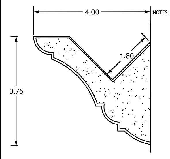
CONSTRUCTED FROM AN EXTRUDED POLYSTYRENE BASE, A FLEXIBLE CEMENTITOUS BASECOAT AND A REVOLUTIONARY, SMOOTH POLYMER MODIFIED PLASTER FINISH.
