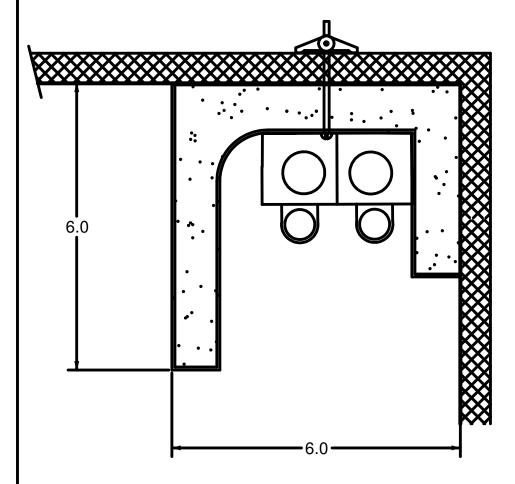
MATERIAL: CONSTRUCTED FROM AN EXTRUDED POLYSTYRENE BASE, A FLEXIBLE CEMENTITOUS BASECOAT AND A REVOLUTIONARY, SMOOTH POLYMER MODIFIED PLASTER FINISH.
